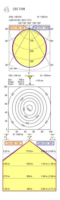
light source LED work equipment electronic transformer connected load 100-240 V, 50/60 Hz; secondary 24 V, DC power consumption env. 27 W luminous flux approx. 1.300 lm luminous efficiency approx. 54 lm/W light type/-color D50 standard light; cold white colour temperatur approx. 5.000 K color rendering index CRI > 95; R9 > 85 light distribution direct
